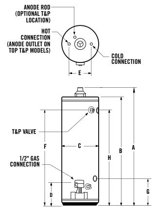
**Maximum Hydrostatic Working Pressure: 150 PSI**
