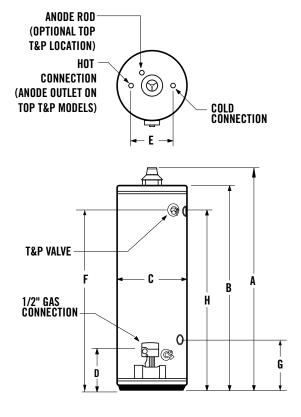
Maximum Hydrostatic Working Pressure: 150 PSI
