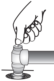
Figure 6. Testing the Temperature-Pressure Relief Valve
