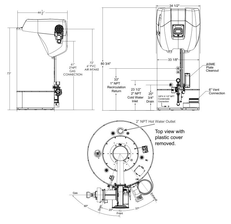
Electrical characteristics-120V-60Hz A.C., 5.0 A "A" in model represents ASME construction Propane gas models available Dimensions and specifications subject to change without notice in accordance with our policy of continuous product improvement.
