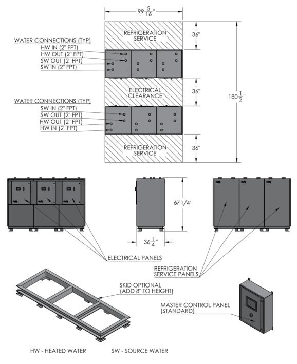
NOTE: 36" electrical service clearance per NEC 110.26(A)(1) Working Spaces for "Condition 1." Check with local codes for additional requirements.
