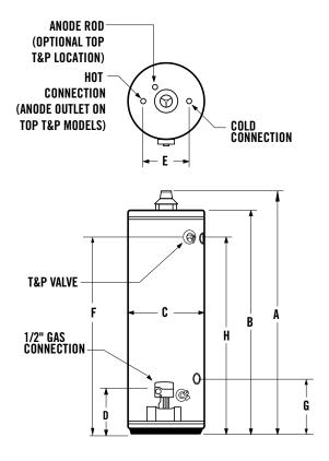
Maximum Hydrostatic Working Pressure: 150 PSI
