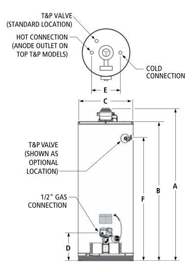
Maximum Hydrostatic Working Pressure: 150 PSI.
