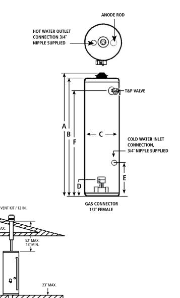
\*Inlet air pipe included 3"diameter for 30 gallon and 40 gallon. 4" diameter for 50 gallon
