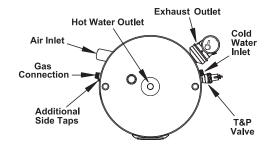
Top Outlet: 1" NPT Side Inlet: 1" NPT
