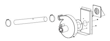
The blower assembly functions by pulling in air from outside the unit to supply to the burner assembly for proper combustion. The blower pushes the air through the burner assembly and heat exchanger where the flue gases then exit the exhaust system assembly, see Figure 8.
