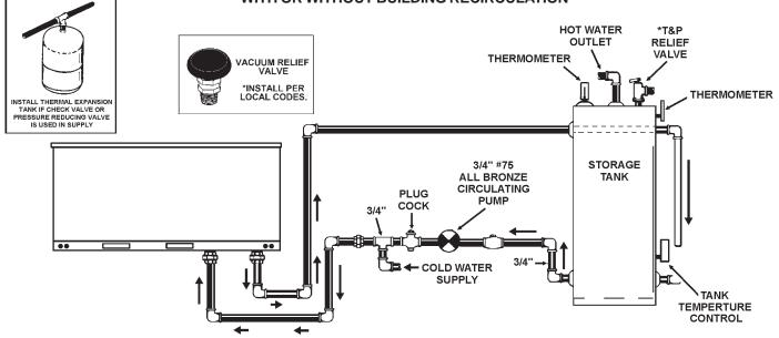
CAUTION: IF BUILDING COLD WATER SUPPLY HAS A BACK-FLOW PREVENTER, CHECK VALVE OR WATER METER WITH CHECK VALVE PROVISIONS FOR THERMAL EXPANSION OF WATER IN THE HOT WATER SYSTEM MUST BE PROVIDED
