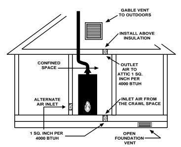
ALL AIR FROM OUTDOORS: INLET AIR FROM VENTILATED CRAWL SPACE/OUTLET AIR TO VENTILATED ATTIC
