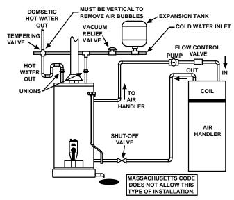
TYPICAL TEMPERING VALVE INSTALLATION COMBINATION SPACE HEATING/POTABLE WATER HEATING SYSTEM
