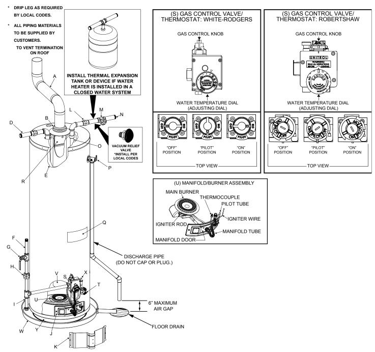
\*NOTE: Round igniter button configuration shown. Igniter button configuration and location may vary. Reference the lighting instructions on the water heater for use/location of the igniter button.
