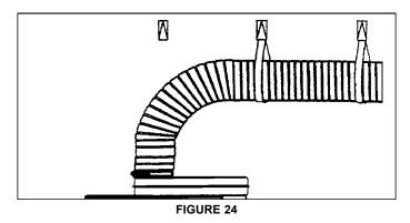
Check the level or slope of the venting again, and adjust if required.
