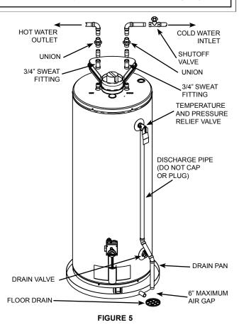
Figure 5 shows the typical attachment of the water piping to the water heater. The water heater is equipped with 3/4" NPT water connections.
