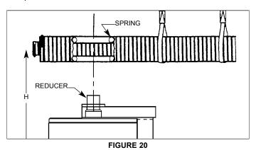
Bend both the corrugated tubes toward the water heater's flue connection.
