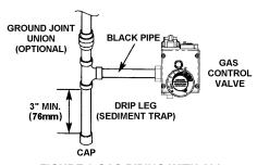
FIGURE 9 GAS PIPING WITH ALL BLACK IRON PIPE TO GAS CONTROL.
