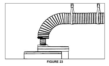
Apply hi-temp red silicone (included) around the collar on air manifold box. Pull corrugated vent tube all the way on to collar and secure with one sheet metal screw (approx. 3/4 in. (19mm) up from edge of vent tube. Pull gear clamp past screw and tighten.
