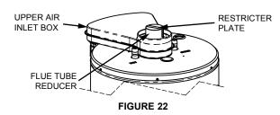
Pull and connect the inner corrugated tube to the water heater's flue tube reducer with hi-temp red silicone (included) and gear clamp. Make sure this connection is tight and leak proof.
