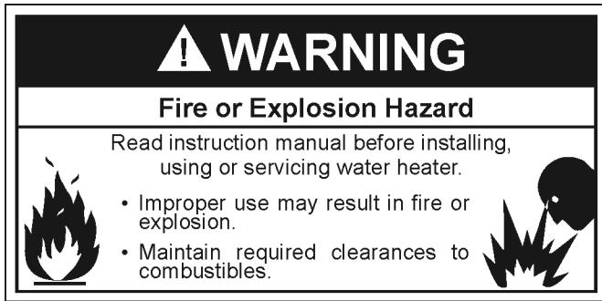
Minimum clearances between the water heater and combustible materials are 0 inch at the sides and rear, 4" (102 mm) at the front, and 6" (153 mm) from the vent pipe. Clearance from the top of the jacket is 12" (305 mm) on most models. Note that a lesser dimension may be allowed on some models, refer to the label attached adjacent to the gas control valve on the water heater, see Figure 3.
