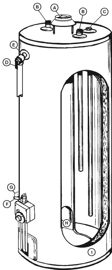
Never use this water heater unless it is completely filled with water to prevent damage to the tank. Water must flow from the hot water faucet before turning "ON" gas to the water heater.
