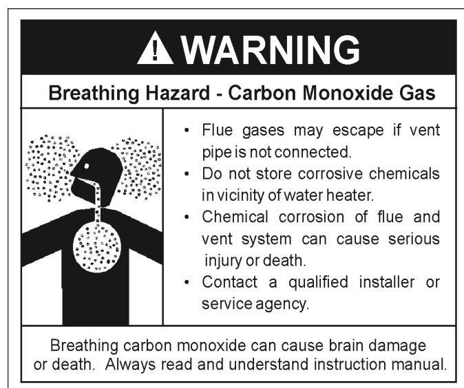
Chemical vapor corrosion of the flue and vent system may occur if air for combustion contains certain chemical vapors. Spray can propellants, cleaning solvents, refrigerator and air conditioner refrigerants, swimming pool chemicals, calcium and sodium chloride, waxes, bleach and process chemicals are typical compounds which are potentially corrosive.
