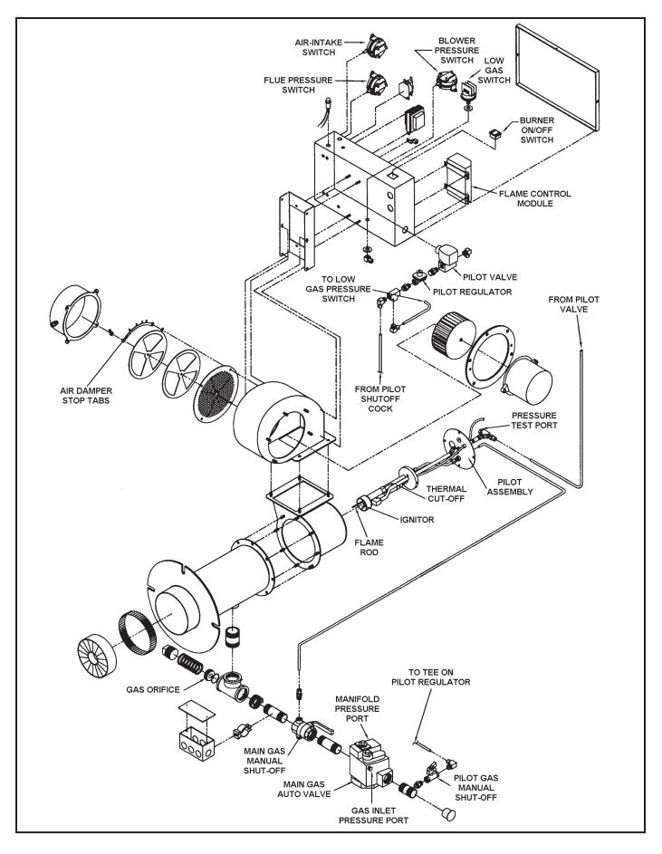
PREMIX LOW NOx BURNER - EXPLODED VIEW FOR GPV MODELS FIGURE 26. For all parts on this burner contact: Wayne Combustion Systems, 801 Glasgow Ave., Fort Wayne, IN 46803
