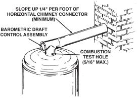
PROPER DRAFT CONTROLLER AND VENT PIPE INSTALLATION FIGURE 16.
