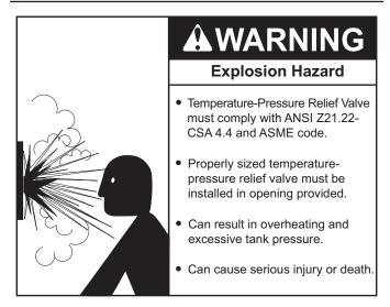
This water heater is provided with a properly rated/sized and certified combination Temperature-Pressure Relief Valve (T&P valve) by the manufacturer. The valve is certified by a nationally recognized testing laboratory that maintains periodic inspection of production of listed equipment of materials as meeting the requirements for Pressure Relief Valves for Hot Water Supply Systems, ANSI Z21.22 • CSA 4.4, and the code requirements of ASME.
