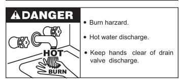
It is recommended that the water heater storage tank be drained and flushed every 6 months to reduce sediment buildup. The water heater should be drained if being shut down during freezing temperatures. See Features And Components in this manual for the location of the water heater components described below.
