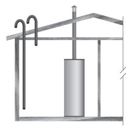
The confined space shall be provided with two permanent vertical ducts, one commencing within 12 inches (300 mm) of the top and one commencing within 12 inches (300 mm) of the bottom of the enclosure. The vertical ducts shall communicate directly with the outdoors. See Figure 14.
