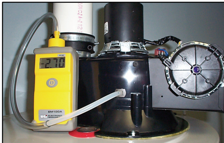
Taking an air pressure reading
