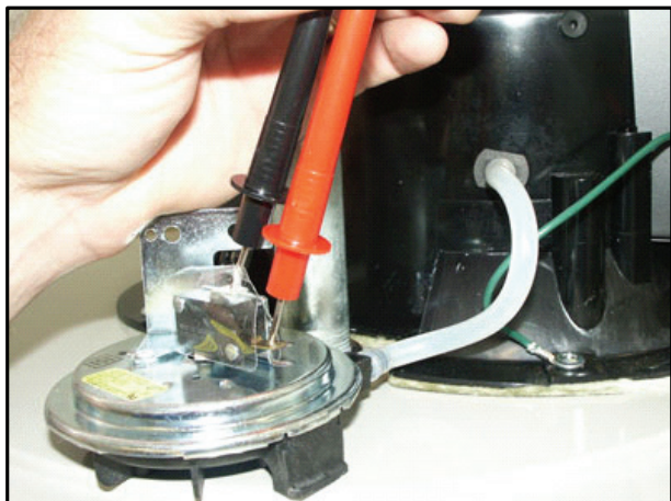
Continuity test with ohm meter
