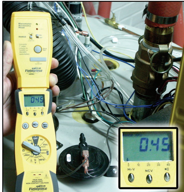
Blocked Exhaust Switch Pressure Test Cyclone - BTH 120 - 250 Models
