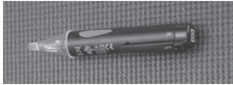
Figure 25 - Non-Contact Circuit Tester
