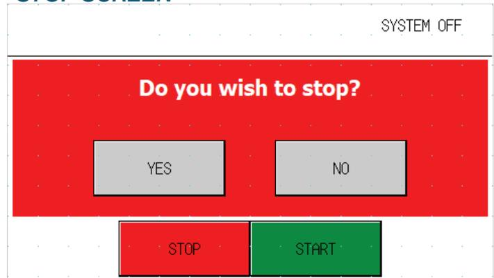
The stop screen will pop up as a confirmation whenever the “STOP” button on any screen is pressed.
