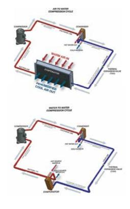
It's more efficient, and less expensive, to move heat than create it. State commercial air and water source heat pumps draw heat energy from ambient air or available source water to provide a more efficient, zero-emissions solution for your water heating needs.
