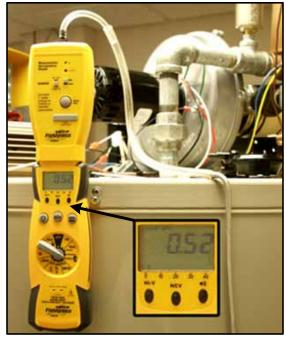
Blocked Exhaust Switch Pressure Test Cyclone - BTH 300/400 Models
