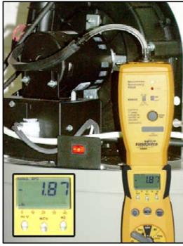
Blocked Vent Switch - Pressure Test Vertex Residential Power Vent Model
