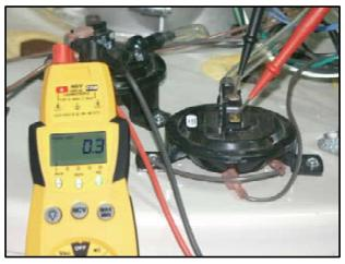
Continuity Test With Ohm Meter BTH 120 - 250 Blocked Exhaust Switch
