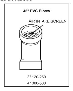
Two 3" or 4" 45° PVC elbows with mesh screens are provided with each unit. Both elbows are to be used in direct vent applications. The screens are provided to keep vermin and large debris from entering the intake air and exhaust vent runs.
