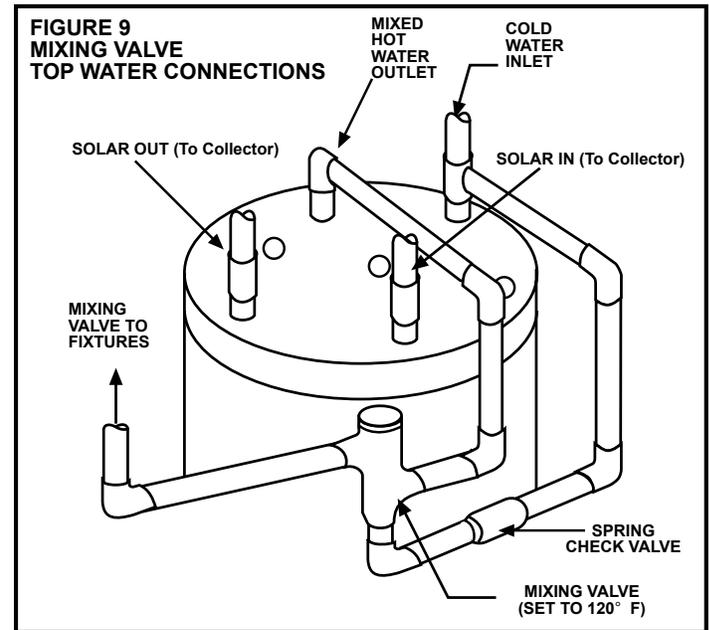
The water supply pressure should not exceed 80 psi. If this occurs, a pressure reducing valve with a bypass should be installed in the cold water inlet line. This should be placed on the supply to the entire house in order to maintain equal hot and cold water pressures.
