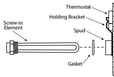
5. Clean the area where the gasket fits to the tank. If you are replacing the bottom element, remove any accumulated sediment on the bottom of the tank.
