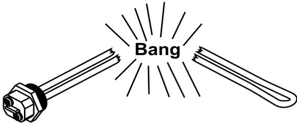
**Notice:** Applying electrical power to elements that are not submerged in water will destroy them. The manufacturer will not warranty any elements damaged in this manner.
