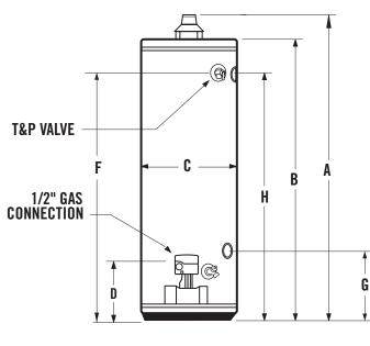
**Maximum Hydrostatic Working Pressure: 150 PSI**
