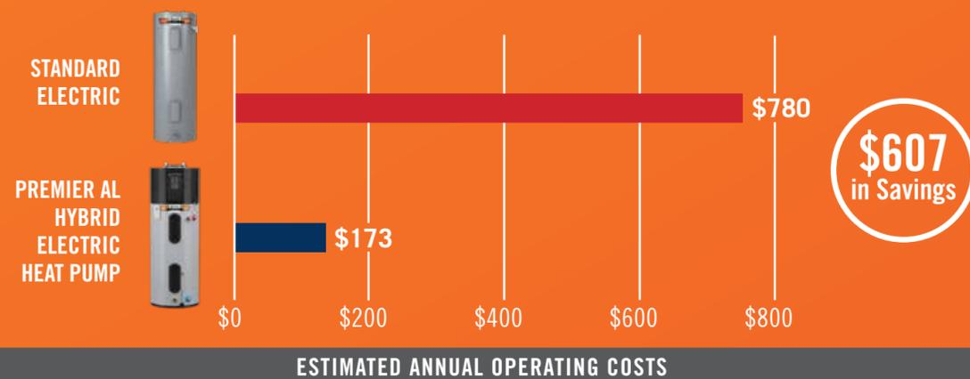
Comparing 66-gallon Premier AL heat pump against pre-2015 similarly-sized standard electric using DOE EF to UEF conversion rates and \$0.14 per kWh electricity cost. Savings may vary.
